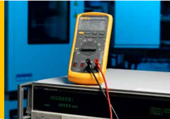
A meter, straight out of the test chamber at -20 °C, measuring 1,000 Volts AC1KHz while covered with ice.
